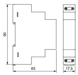
Module T924P1 is a passive separator of  $4 \div 20 \text{mA}$  signal (it functions in fact from almost 0 mA to about 25 mA where internal limiting circuit turns on). Factory test isolation voltage equals 2 kV.
